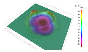
3D surface measurement of a steel specimen after five impacts by the high velocity particle impact test at a temperature of -60°C.
