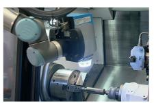
The sensor then moves on to the workpiece and measures its roughness to verify surface quality. Then the robot arm returns into its original position. All measurements are carried out without
