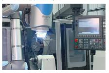
and a further signal sets the Cobot in motion. The robot arm with 3D measuring sensor is automatically manipulated into the lathe.
