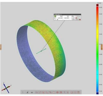
Inspection of diameter and cylindricity
