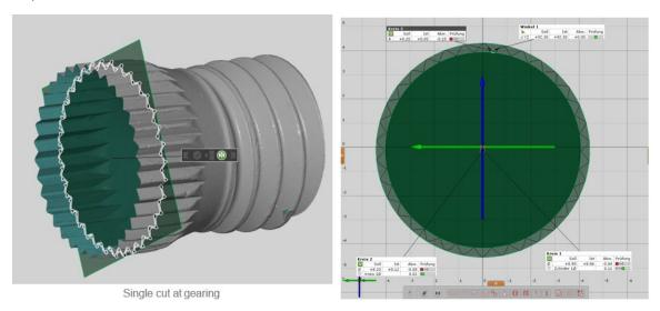
Using the same 3D model, a feature of optical metrology is that all dimensional information can be extracted without additional probing we then move to the measurement position B and display the 3D model in real colour and pseudo colour related to height, displayed below and measurements of angles, radii and distances made.
