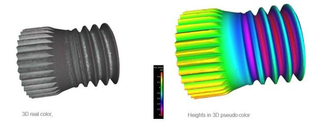
Using the Alicona Inspect Module it is then possible to display and measure, at area A, the profile geometry as shown below describing, on the right, OD, ID, circumscribed element and inscribed element
