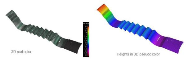
Sample 2 - Measurement area B - Alicona Sample 2 - Measurement area B - Alicona Inspect - Fitting of cylinder Inspect - Pattern construction
