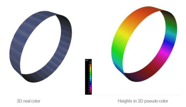
A cylinder is fitted to the dataset to describe diameter and cylindricity as shown below.
