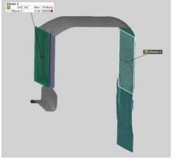
Inspection of parallelism between plane 1 and plane 2
