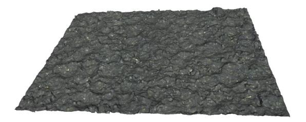
Figure 2: 3D measurement, from the InfiniteFocus of the hot plate surface in true color. The hot plates warm up the cover film before sealing it onto the base foil. Alicona enables Uhlmann to determine the surface finish parameters (Sa, Sz) and material parameters (Sk, Spk).
