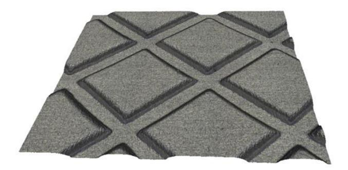
Figure 3; 3D measurement of a blister sealing area in true color
