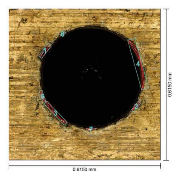
7 Identified burrs identified with the defect detection module
