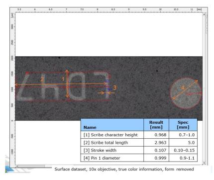
Using the same data, the profile of the characters can be measured in 3D by extracting a profile line across the surface as shown below
