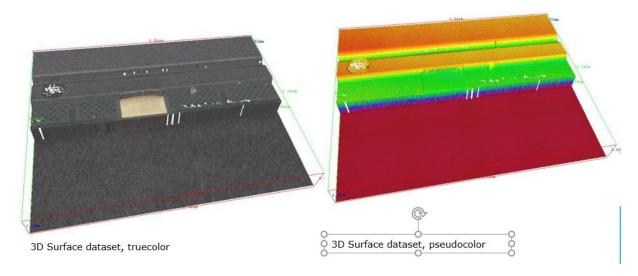
Using the profile measurement, the warpage can then be measured as shown below.
