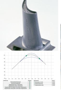
Even the smallest form deviations are measured traceably. The evaluation is performed automatically and according to common industry standards, e.g. ASME.
