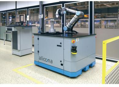
Cobots consist of a collaborative 6-axis robot and a high-resolution optical 3D measuring sensor and are a popular measuring device for production-integrated quality assurance.
