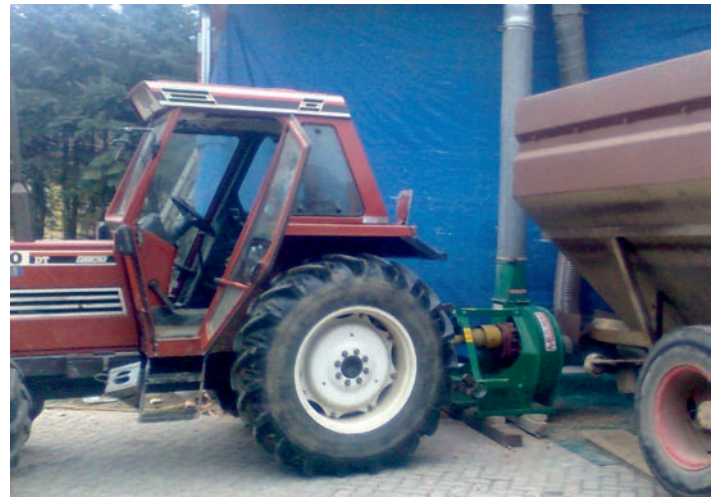
Tractor blower with suction mechanism – container feeding
