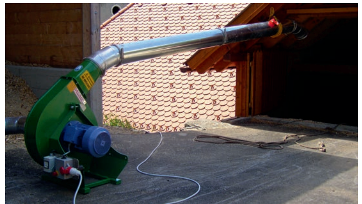
Suction blower with suction hose – can be used anywhere
