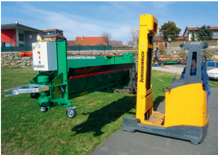
Trough-type blower can be handled with forklift – simple to load
