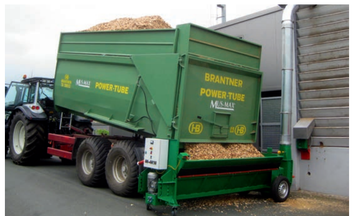
Trough-type blower with electric motor – ideal up to 30 m³/h
