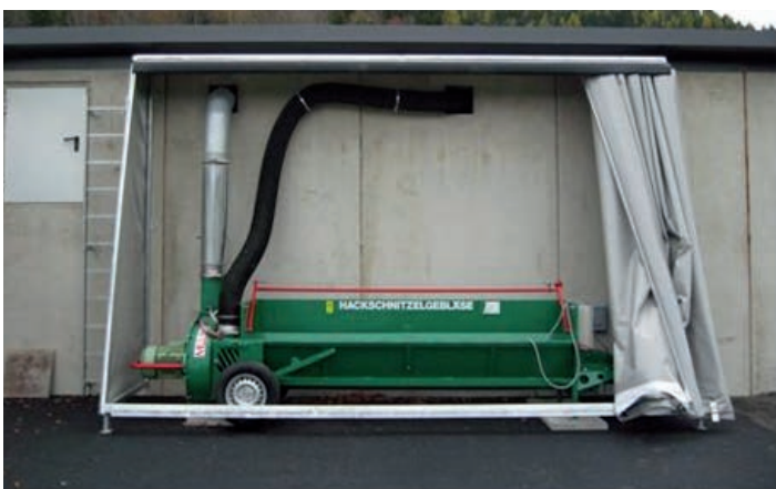
Trough-type blower with return suction mechanism – for dust-free working
