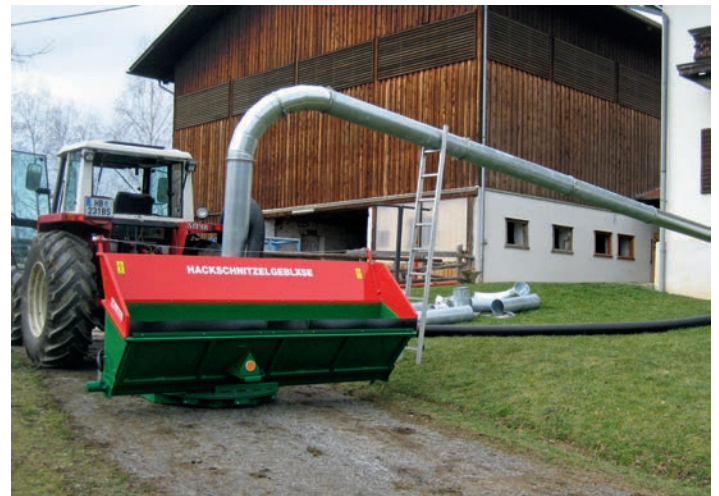
Tractor blower with swivel-mounted trough – high output
