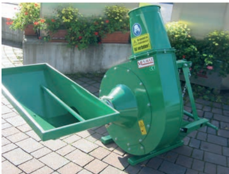
Air can also be drawn back from the hopper.
