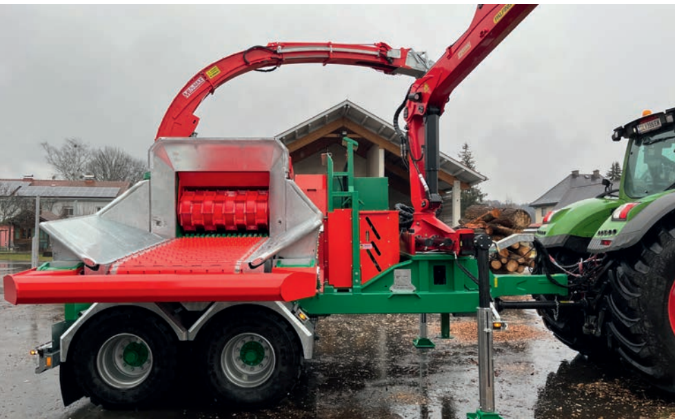
Infeed system on model WT 11L Z
