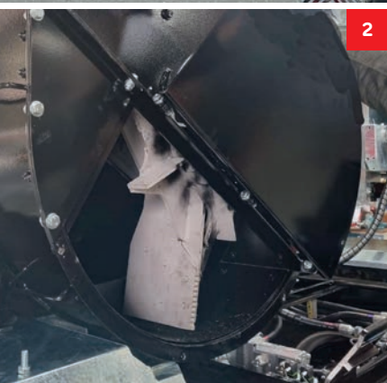
1. Hydraulic blower with swivelling blower cover 2. Mechanical blower (optionally with industrial freewheel) 3. New MUS-MAX high-performance fan blade
